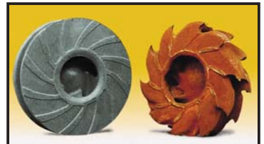
Warman Standard Impellers - new and after five million tonnes - and at a loss of only 5% in efficiency from beginning to end
